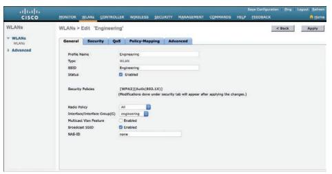
Figure 4-31 Configuring the General WLAN Parameters
