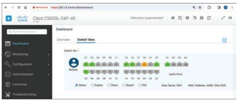
Figure 4-8 Cisco Switch Web Interface Dashboard: Switch View
