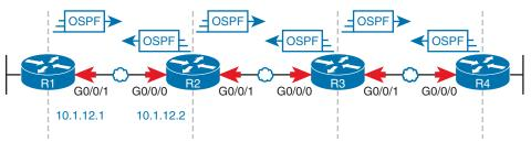
Figure 8-2 OSPF Message Flow Between Routers R1 and R2
